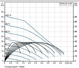
Pumped liquid = Water Liquid temperature during operation = 20 °C Density = 998.2 kg/m<sup>3</sup>
