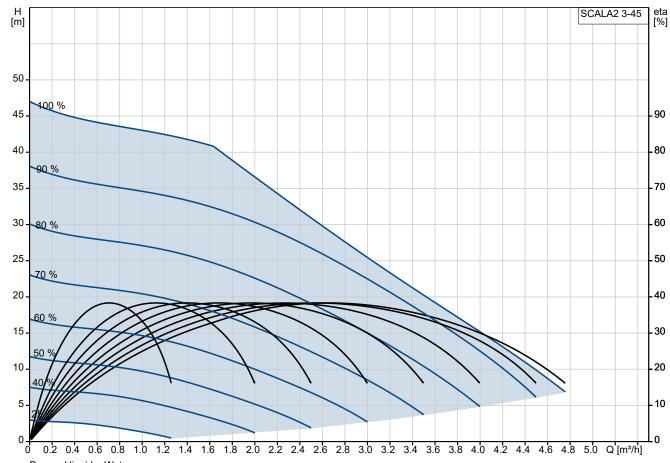
Pumped liquid = Water Liquid temperature during operation = 20 °C Density = 998.2 kg/m³
